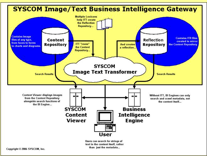
The diagram above illustrates the logical structure of an IBIG installation. While it is possible to build an environment that physically mirrors this structure, it is not necessary. Depending on the needs of the organization, SYSCOM can customize IBIG in a number of ways.
